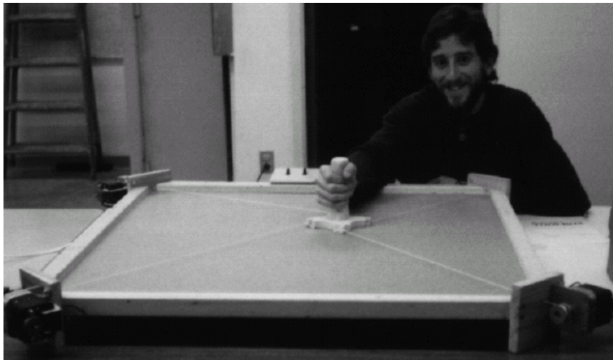
Figure 2-10: Four-cable planar “cable-suspended haptic interface”
